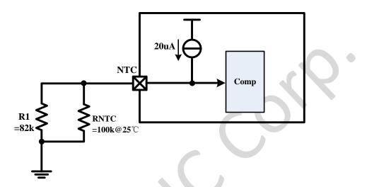
IP2723T support NTC function used for temperature detection. NTC pin output 20uA current then detect the voltage on NTC pin to determine the present temperature.
