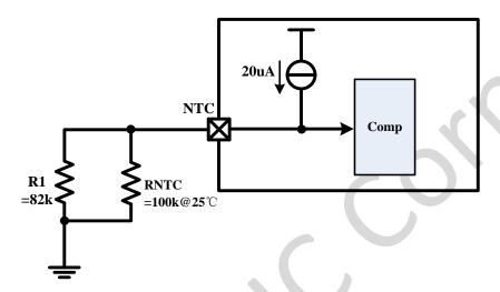
IP2723TH support NTC function used for temperature detection. NTC pin output 20uA current then detect the voltage on NTC pin to determine the present temperature.
