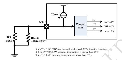
IP2163H\_AT integrates NTC temperature sensitive resistor detection, and supports abnormal temperature indication on FA pin. NTC and FA are multiplexed with CSN and CSP function on Pin 1 and Pin 2, only one function is enabled at the same time.
