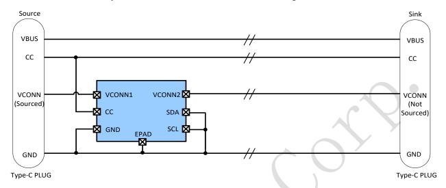
Passive Cable : Electronically Marked Cable with SOP' at both ends(with VCONN not connected through the cable)
