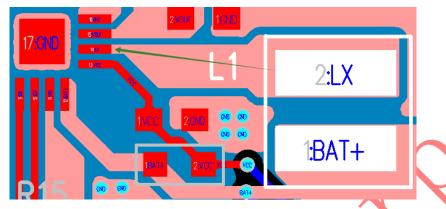
6. It is forbidden to layout any other networks wire under the 5521 chip. Only GND vias need to be drilled under the EPAD:
